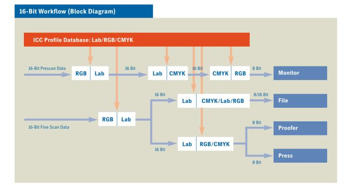
Multifunctionality is a must • Color scanning and redigitization for the digital workflow are essential for today's prepress. Specialized Copydot scanners are expensive and no-one can say, how long they will be required. You should therefore invest in a scanner that can handle both.
